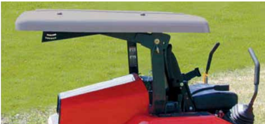
Folded, ready for transportation. Folds flat to folded roll bar.
