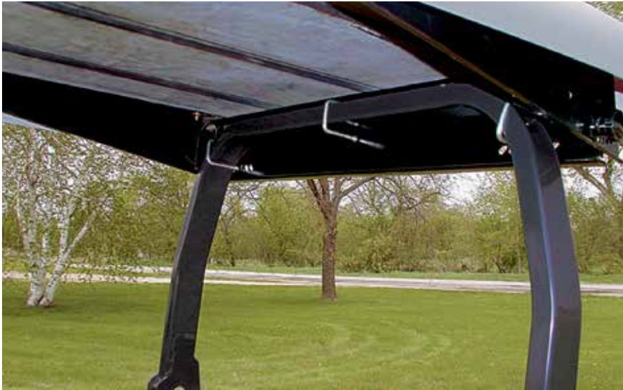
Plastic sunshade clamps to roll bar without drilling.
