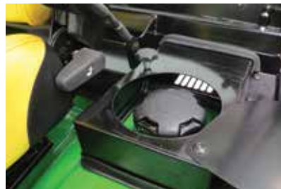
Vented fuel fill access door
