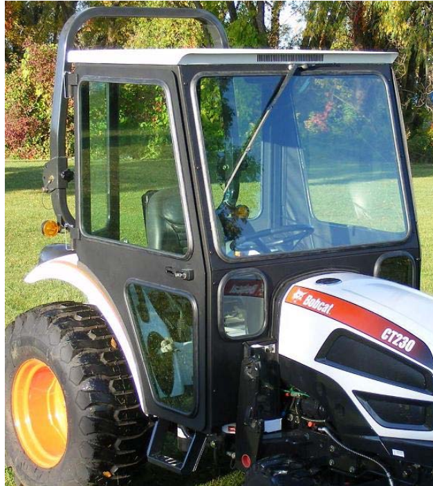
A-11718 CAB FRAME WITH A-11635 BOBCAT ROOF KIT ON BOBCAT 200 SERIES TRACTOR (SHOWN WITH OPTIONAL HARD DOORS)
