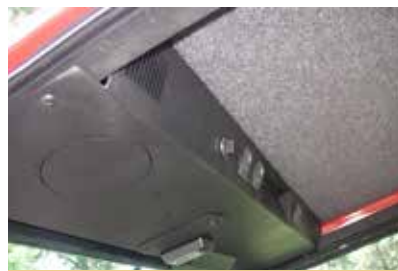
Headliner with fuse block, dome light and power port
