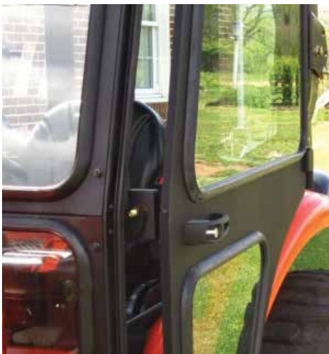
Increased ventilation with door hold-open feature
